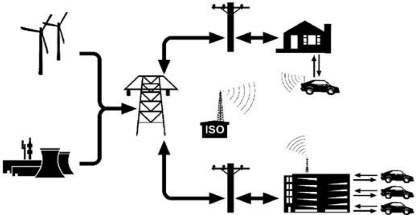
V2G: *Prosumer vision*: storage V2G helps RE integration in microgrid; enhancing acceptance and limiting transmission
