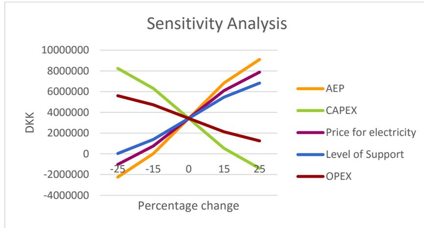
Figure 6-7 Sensitivity Analysis of the 3.0MW wind turbine
