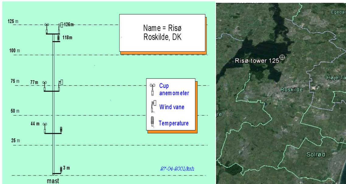
Figure 3-2. The meteorological mast sited at Risø campus.
