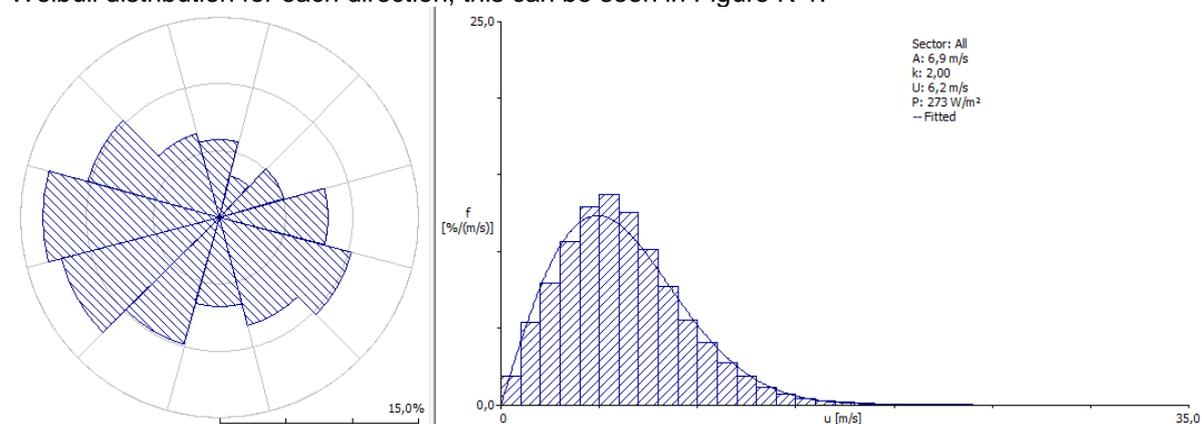
Figure K-1 Imported wind data, height 44m a.g.l. both the direction and the mean wind speed can be seen.
