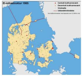
Figure N-1 The grid system in Denmark in 1985 A few large centralized power plants producing electricity in Denmark. From (The Danish Energy Agency 2014 B)
