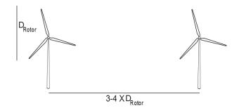
Figure 3-4 Recommend distance between the wind turbines in a Danish wind farm. To decrease the wake impact on the EAP the distance between two wind turbines should be 3-4 times the rotor diameter. This is the recommended distance; however, a higher distance can be preferred, to decrease the wake impact further. Data from (The Danish Energy Agency 2009 A)
