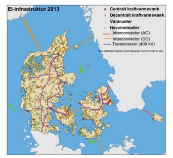
Figure N-9-6 The grid system in Denmark 2013 Many small decentralize power plants producing electricity and heat in Denmark. From (The Danish Energy Agency 2014 B)
