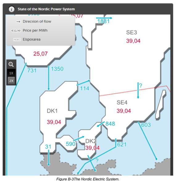
The Nordic electricity connections, across the national borders. The level figure is from October 13, 2015, 09.40. The level of electricity transfer and cost can be seen at each electricity system. Figure from (Energinet 2015 A).
