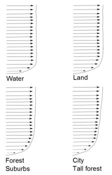
Figure J-2 Roughness Impact on the Wind Profile.
