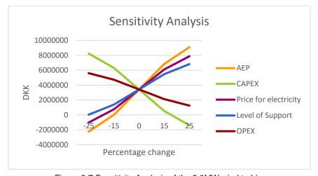
Figure 6-7 Sensitivity Analysis of the 3.0MW wind turbine Feasibility calculations for a Siemens wind turbine with a hub height of 127.5m, where the different variables are AEP, level of CAPEX and OPEX, price for the electricity and support.
