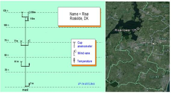
Figure 3-2. The meteorological mast sited at Risø campus.
