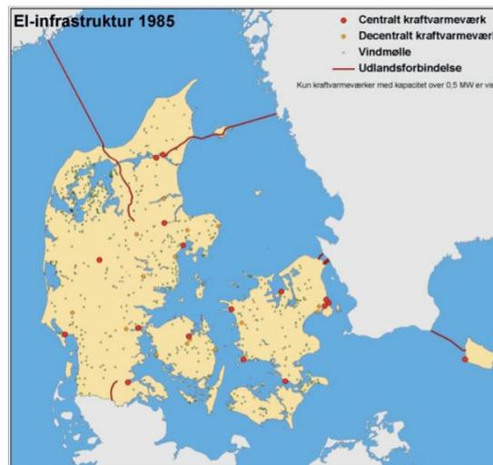
Figure N-1 The grid system in Denmark in 1985
