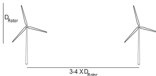
*Figure 3-4 Recommend distance between the wind turbines in a Danish wind farm.*
