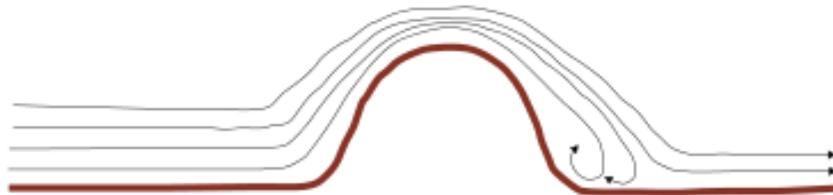
Figure 3-1 Wind flow over a steep hill.
