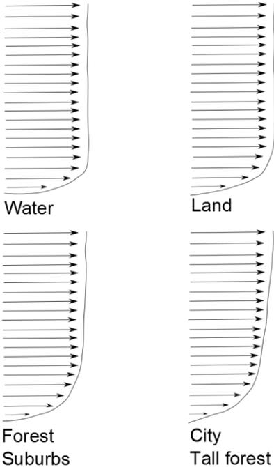
Figure J-2 Roughness Impact on the Wind Profile.
